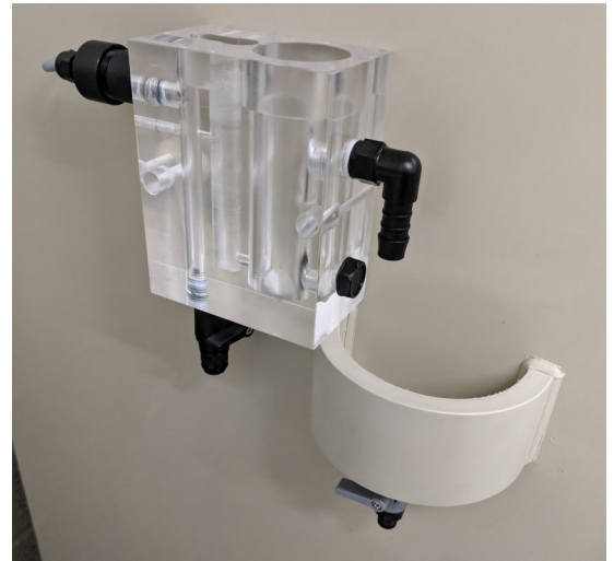
An example of an installation with an air break in the sample outlet
